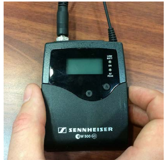
Opening the front panel of the lapel microphone
