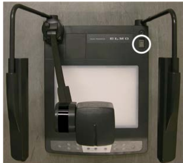
Power switch location
